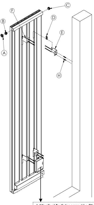
"Attention! Radiator cannot be fitted upside down. The power cable and control modem are down side. Otherwise, product can has breakdown and will be considered out of warranty."
